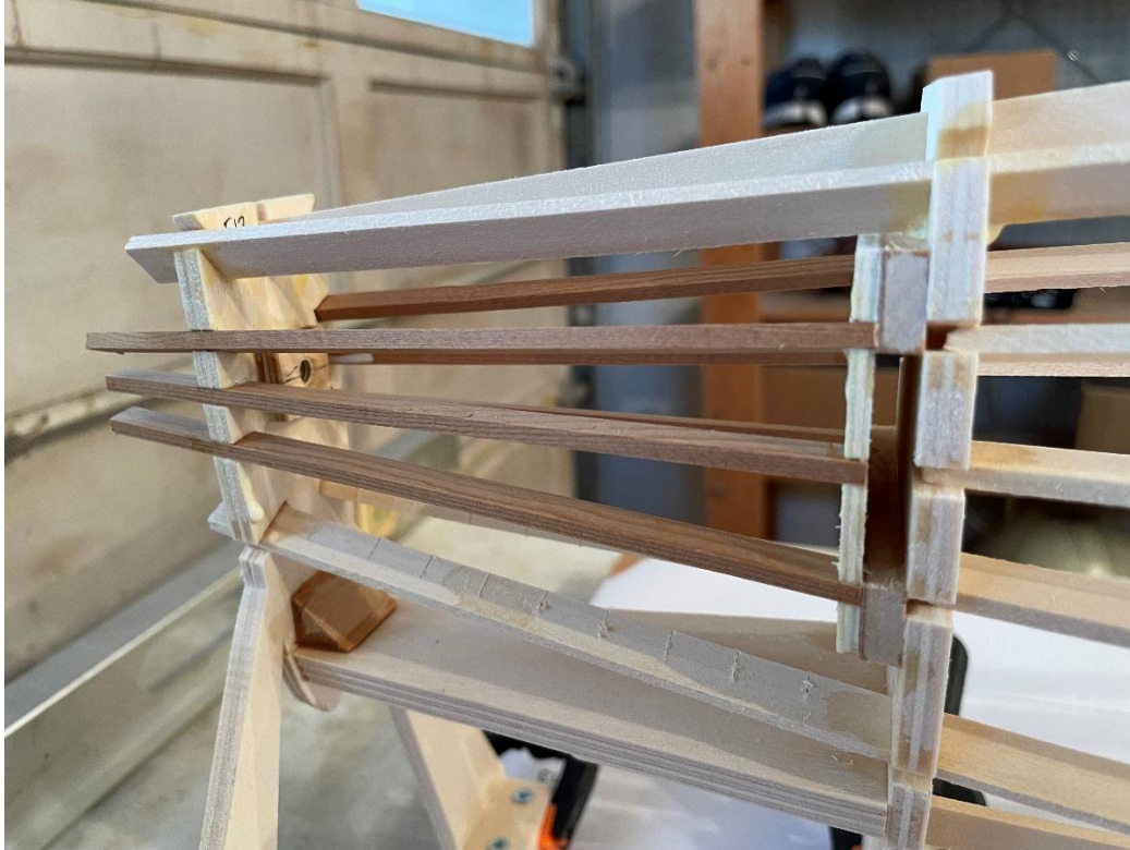
The wing tube socket and SW3 ribs are in place to ensure correct alignment. They are NOT glued.
