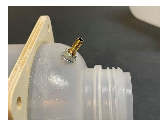
Drill (2) 3/16" holes from inside the cap. Install brass nipples as before.
