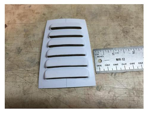
Position the louvers on-center at the 11am and 1pm position, locating the edge of the first louver about one inch forward of F1. Secure with masking tape. Do the same at the 7a and 5p positions at the bottom.
