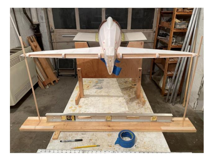
Be sure to mask off any part of the fuselage where glue squeezed out might drip.
