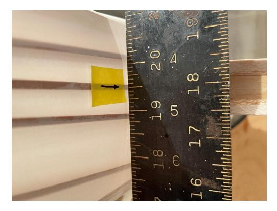
Rig up any suitable method to support the stabilizer at the tips. If you are very careful, you can simply use two pieces of basswood wing spar material and drill 1/16" holes at the calculated stabilizer height distance and pin it to the tip.
