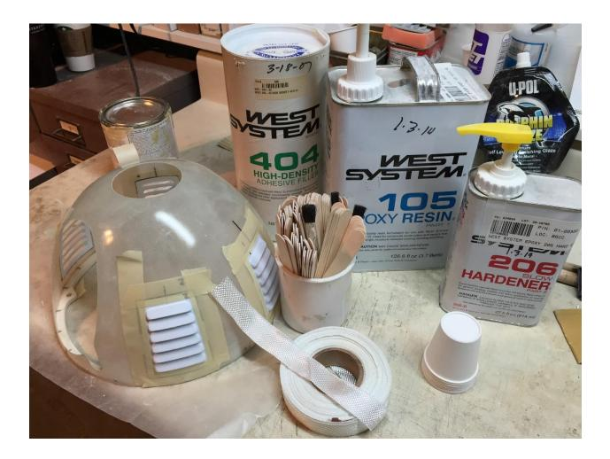
After the resin has cured, fill the seams with auto body filler as needed and sand to a smooth finish.
