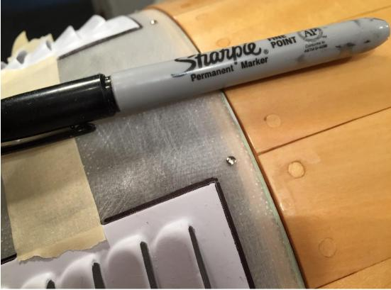
Carefully cut out each section on the cowl to make as closely as possible the outline of the louver section. The reason you do this is so the louvers will appear flush with the surface of the cowl and not look "glued on."
