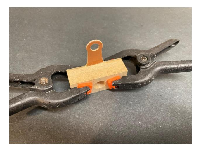
Insert the threaded  $#6-32 \times 1/4$ " x 7/8" nylon axle and temporarily secure forks together with two  $#6-32 \times 1/2$ " socket head screws.
