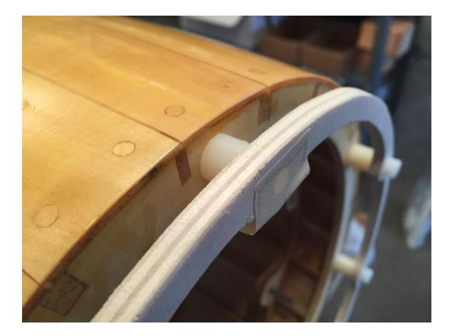
Lightly sand the inside lip of the fiberglass cowl with 100 grit. Mix a small, one ounce batch of epoxy and mix in some filler – enough so it won't run. Apply to the ring only and press the cowl onto the ring. Rotate just a little to spread the epoxy mix. Make sure that the cowl is aligned exactly where you want it.
