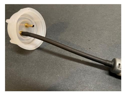
Mount the fuel tank on the right and the smoke on the left as seen from the cockpit. Complete all internal tank plumbing and screw the caps on tightly. Mark the location of each nipple on the caps so you can orient the tanks correctly during installation. For example: I for in, and O for out.
