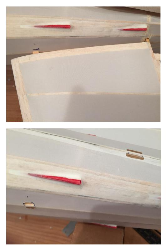
Cut the openings, but don't cut away more than necessary. The flight loads on the tail are relatively light. Virtually all the load on the stabilizer and fin are carried by the 3/16" basswood spars. The tabs just hold the leading edges in place.
