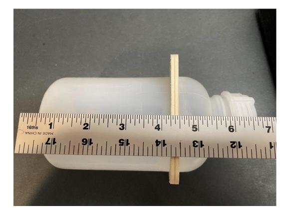
Locate the overflow nipple about  $45^{\circ}$  and on center. Drill a 3/16'' hole. Make sure that no debris remains inside the tank.
