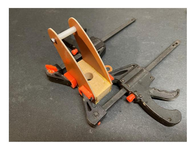
Glue 1/4" balsa sides to the forks. Also fill in the front and rear with 1/4" scrap. Shape with 60 grit and finish with 100 grit sandpaper.
