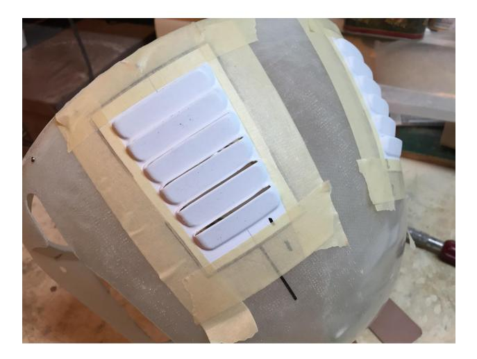
Secure the louver sections from inside the cowl with one inch fiberglass tape and epoxy resin. It is usually advisable to mix in some #404 high density filler to make the resin thicker and prevent the resin from running.
