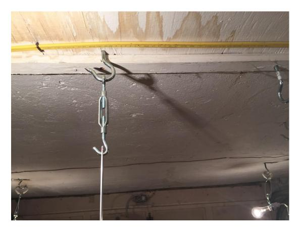
The model has been suspended with  $1/16'' \ge 1/2''$  aluminum bar stock. The turnbuckles are not necessary but work very well if minor vertical adjustments are needed to keep the wings level.
