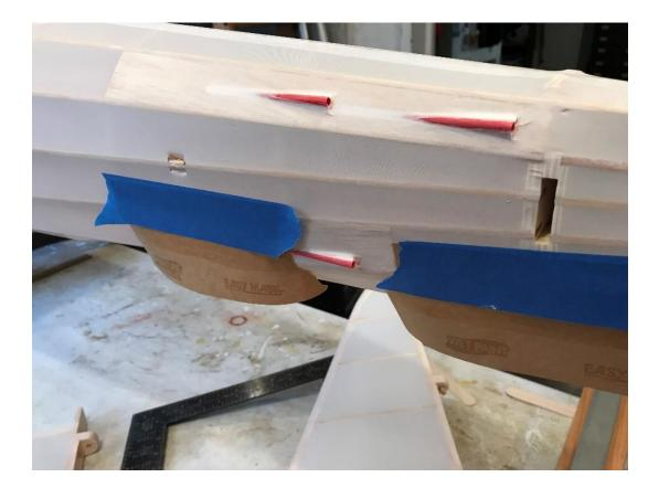
Gluing the stabilizer to the fuselage is straight forward once you are set up and ready. Use Titebond. Titebond glue will begin to "grab" within just a few minutes. It means you only have one chance to do it right. Dry fit to be certain the glue up will go as planned.
