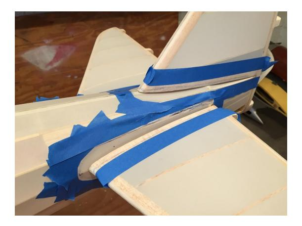
Spread lite spackle. Scrape and shape with the forming disk. Work one section at a time. Form the "first pass" as best you can. As the spackle begins to dry, it becomes easier to scrape into the shape you want and does not so easily pull away. It is easiest to take light passes working toward the center from the edges.
