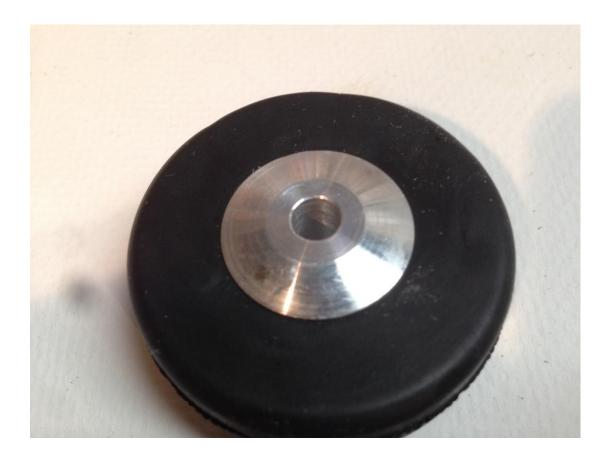
Upon final assembly (after painting), the tail wheel is attached as shown on the fuselage drawing using the parts shown in this picture. The tail wheel will be supported and turn freely on a nylon axle.
