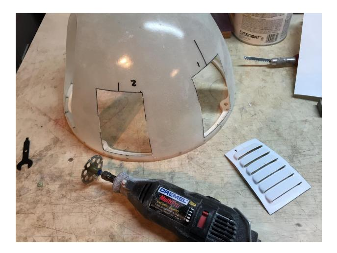
Tape each louver section to the cowl with masking tape. The idea is to tape each section so that the exposed surface is the same as the cowl. Done this way, there should be a minimum amount of filling and sanding necessary. When done properly, the louvers will look like they are part of the cowl –not something that was added. Very realistic
