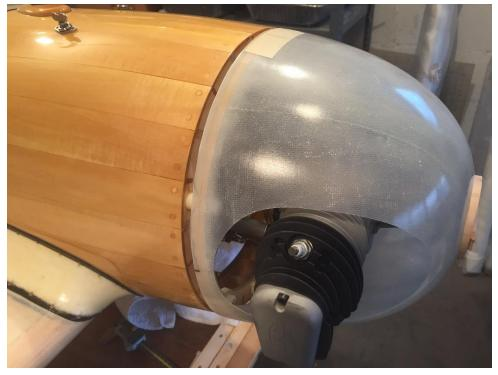
The cowl has now been trimmed and mounted to F1 with four ¼-20 X 5/8" nylon cap screws. You will need a long hex driver to mount and remove the cowl.
