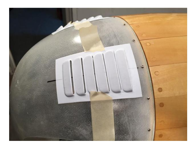
Mark the outline lines of each louvers section with a felt tipped marker. Since the outline of each louver section will be slightly different, make sure to label each section and note its location on the cowl.
