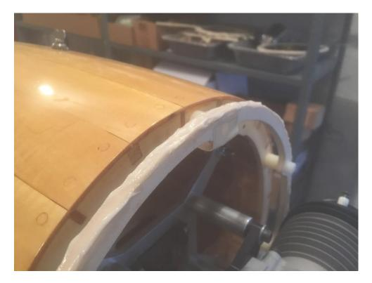
Insert the cowl / propeller hub alignment ring onto the engine hub flush with the face. The ring is made of any material 3/8" thick. Position the cowl onto the ring on-center – 3/16" back from the face of the hub.
