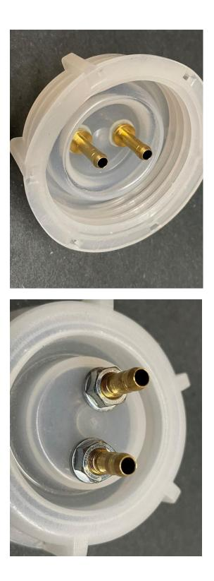
There is no need to use Loctite on the threads. Gas and smoke oil will swell the plastic and create a tight seal.
