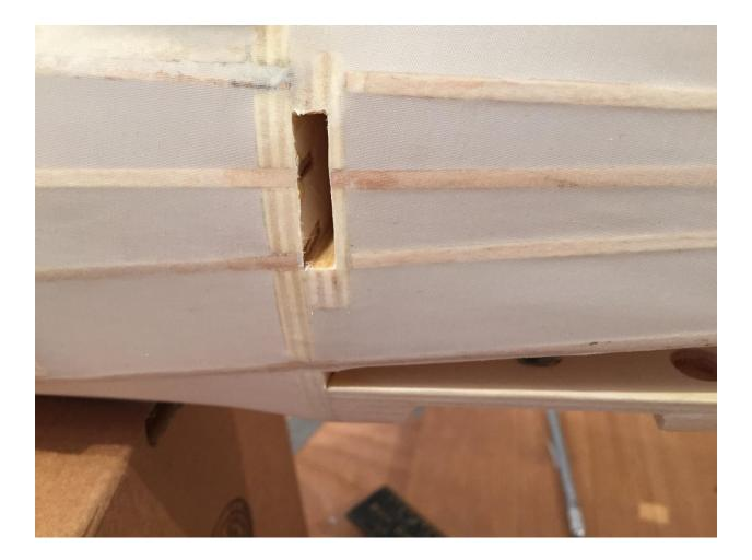
Mark where the forward mounting tabs will enter the fuselage and be glued to the stringers at 9A and 3P.
