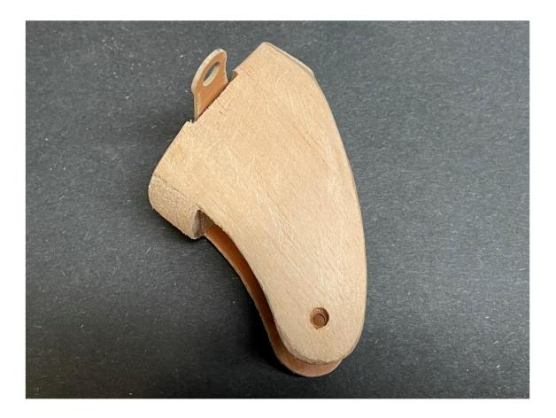
Since balsa is porous, it is best to fill the grain with lite spackle. Just rub it in with your fingers. When dry, finish with 220 sandpaper. Brush on one coat of nitrate dope thinned 1:1. Normally, the tail wheel forks will be painted the same color as the fuselage.
