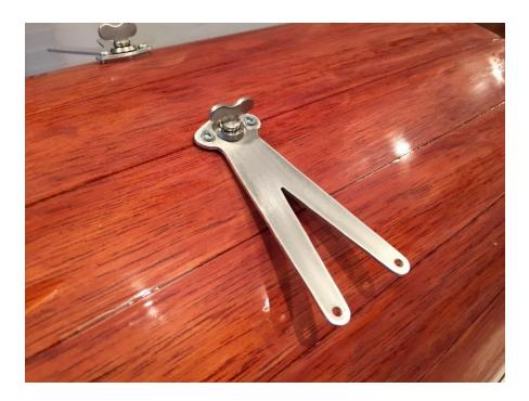
Note: The top wires are properly called "landing wires." The wires under the wing are called "flying wires." Note that the brackets are not symmetrical.
