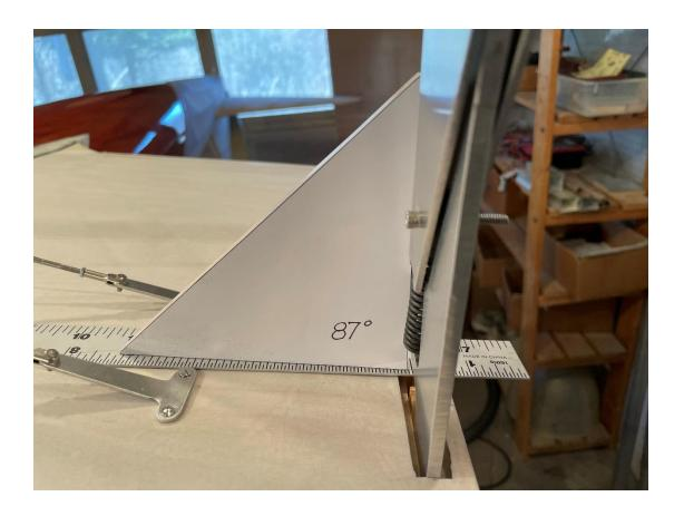
Leave the stretcher in place and under tension while adjusting the wires that attach to the wing panels.
